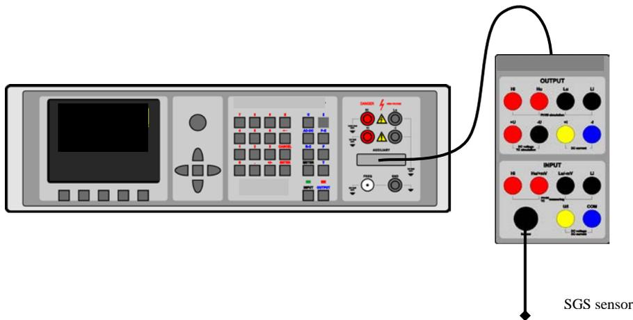
Connection of the sensor to SENSOR connector
