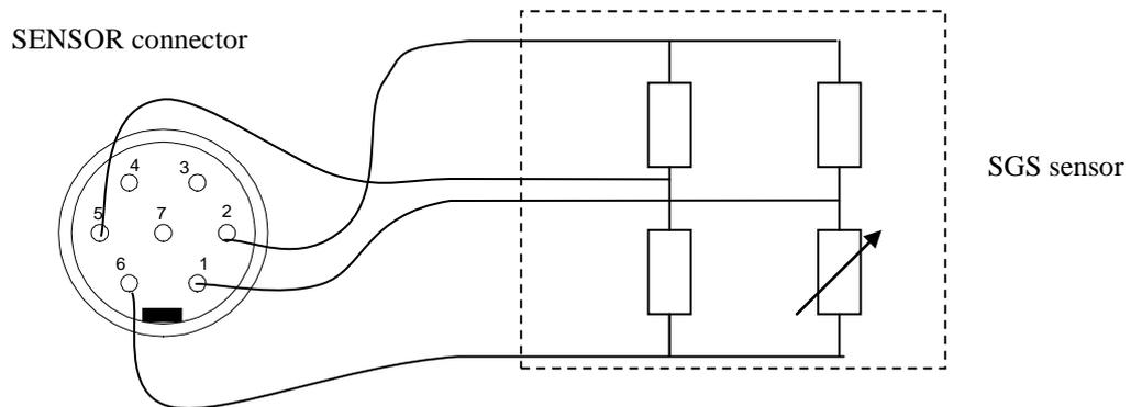
Meaning of pins of SENSOR connector:
