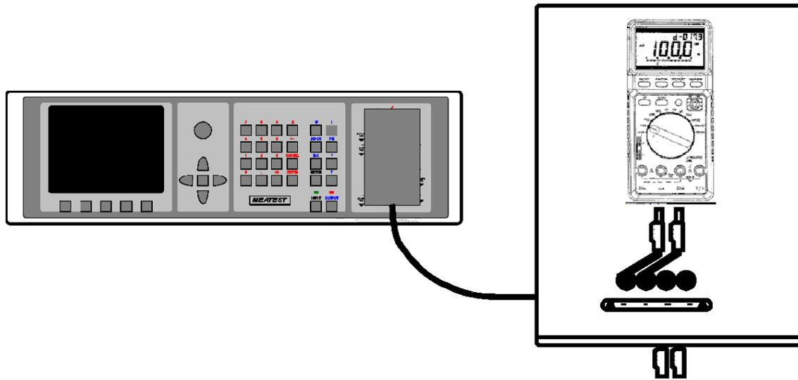
Optional current coil can extend the calibrator's current range to 1000 A. The coil can be used for calibration of both DC and AC ammeters. The clamps of the ammeter must be positioned in angle  $90^\circ$  to the coil. When using the current coil, no steel or other magnetic objects must be present in the vicinity (50 cm) of the current coil, as they would deform the magnetic field and cause big calibration error.
